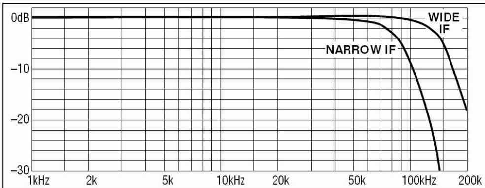
**Figure 4 - Receiver Composite/MPX Frequency Response**
