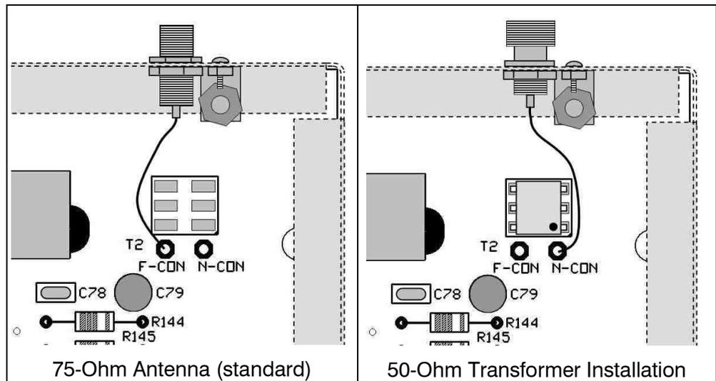
**Figure 6** - Antenna Transformer Option
