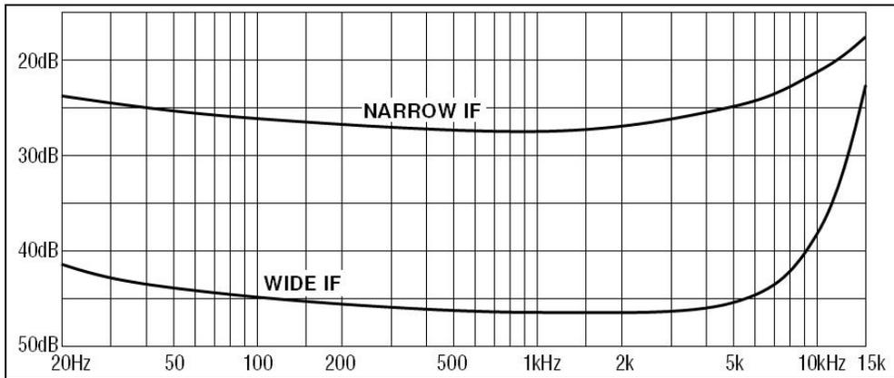
**Figure 3 - Stereo Separation vs. Frequency
