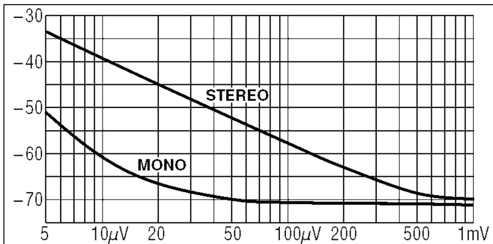
Figure 1 - Receiver Sensitivity - Output Noise vs. RF Input
