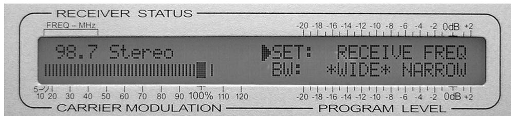
The notation to the right of the frequency readout shows this as a **Stereo** transmission; otherwise the word **Mono** would appear. Signal alarms are also noted in this area. **Lo-Sig** and **A-Loss** alert the operator to a low incoming signal level or loss off program audio. These alarms are pictured here, and their programming is detailed in a subsequent discussion.
